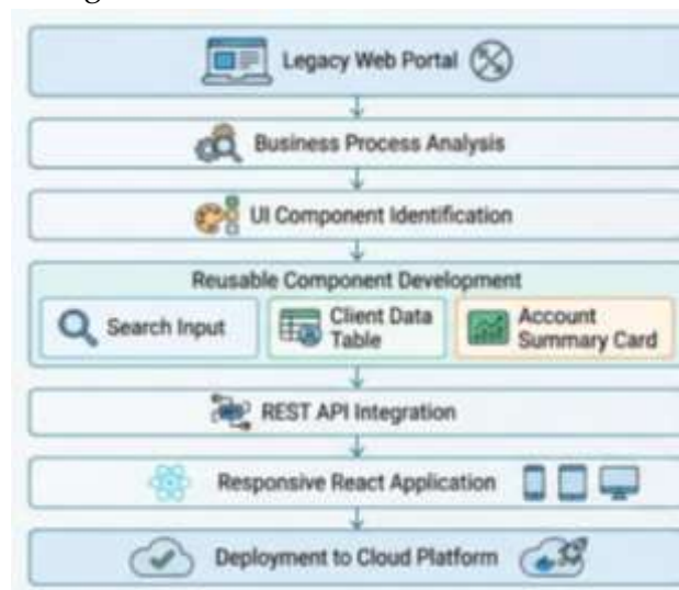
Fig 2 - Front-End Replat forming Workflow
