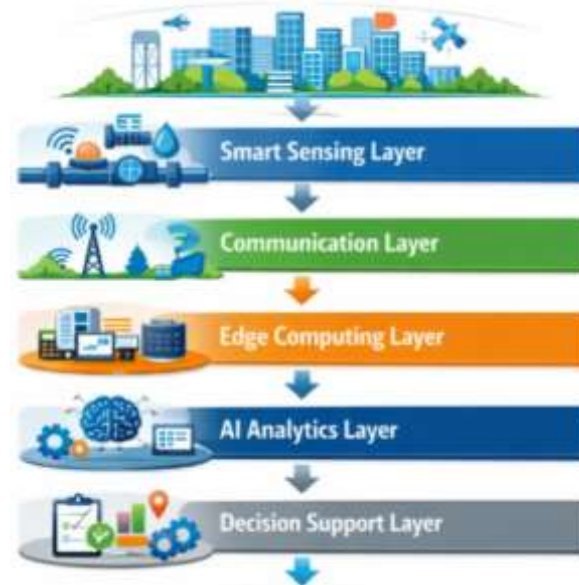
Fig 2 - Proposed AI-Enabled Smart Water Distribution Architecture
