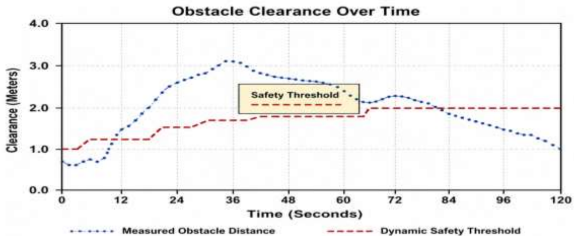
Fig 2- Real-Time Obstacle Distance Clearance Profile And Dynamic Safety Threshold Maintained During A Representative 120-Second Autonomous Inspection Mission.
