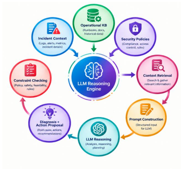
Fig 2 - LLM Reasoning and Retrieval-Augmented Remediation Architecture
