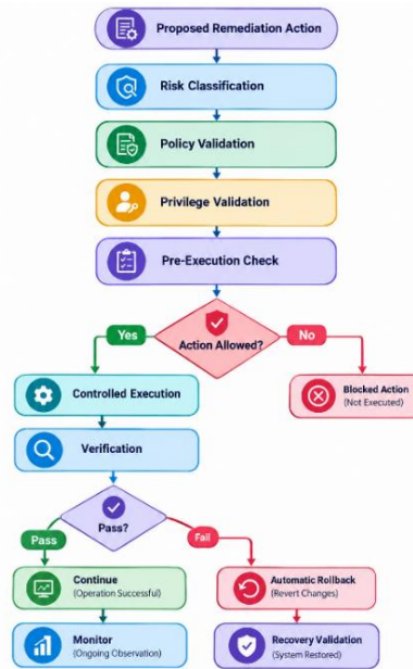
Fig 4 - Safety-Aware Autonomous Remediation Execution Workflow
