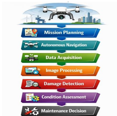
Fig 2 - Proposed Autonomous Drone Inspection Framework
