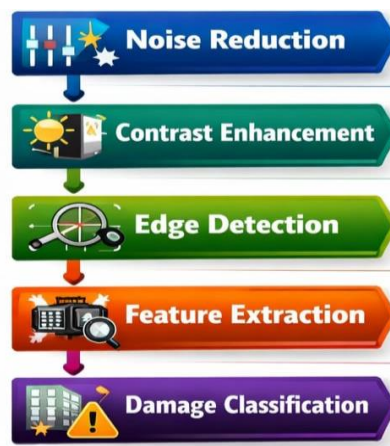
Fig 3 - Image Processing and Damage Detection
